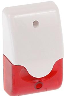
The SV-103 small indoor siren with optical and acoustical signaling is designed for operation in the intruder alarm systems. Optical signaling source are LEDs, and acoustical signaling is generating by piezo transducer.
