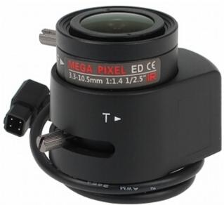
Vari-focal IR corrected lens for day/night megapixel cameras. The lens uses a combination of lenses to compensate the chromatic aberration for infrared wavelengths.
