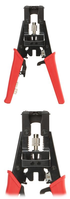
Terminating of BNC compression connectors using a compression tool: :
