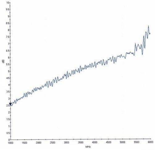
The TRI-LAN-240 cable matching in frequency response:
