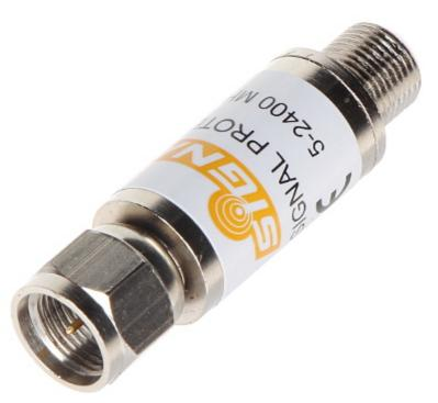
The ZPP-4645F is overvoltage protection of the receivers operating in terrestrial TV full band. It is used for example to protection of: TV receivers, HiFi sets, amplifiers. The device starts to work above 35 V voltage level, in 5-2400 MHz band at attenuation parameter below 0.5 dB. These parameters allow also to work in CATV with return channel applications. Replacement for MSS-01.
