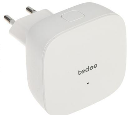
The TEDEE-BRIDGE device operates as a bridge between the Tedee smart lock (Bluetooth interface) and the Internet (Wi-Fi interface).
