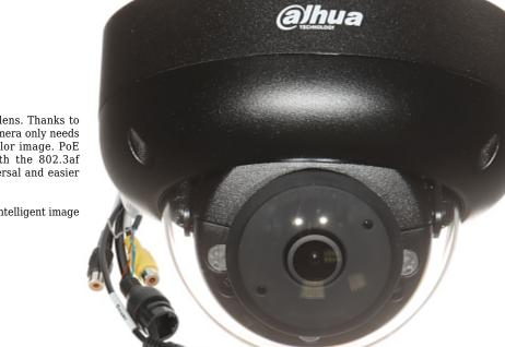
IP camera with "fish eye" wide-angle lens. Thanks to the "Starlight" technology used, the camera only needs very low lighting to obtain a clear color image. PoE powering possibility, compatible with the 802.3af standard makes the device more universal and easier to install.
