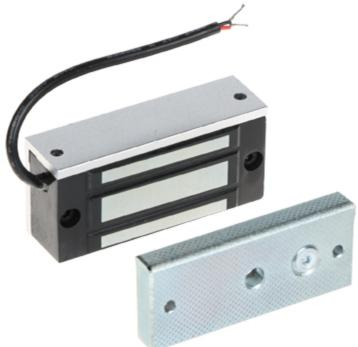
Electromagnetic lock, surface, single. The lock is intended for blocking small wooden, glass or metal doors. Force an entry closed by lock requires the use of force of > 60 kg. It operates reversibly - it is open when power is off. The lock is composed of two elements: electromagnet (usually mounted in the frame) and lock plate (usually mounted in the door). Error free operation of the lock is a result of lack the mechanical elements, which after some time become damaged.
