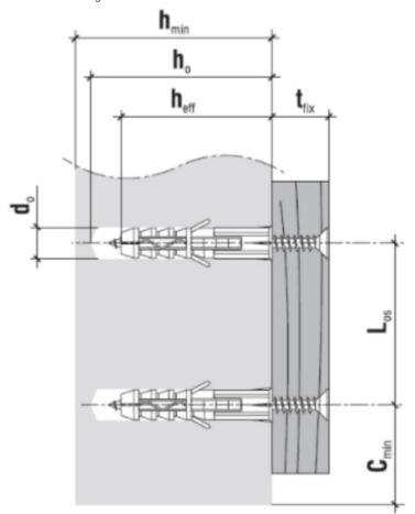
$$\begin{split} & \text{Hole/drill diameter } [d_{\text{o}}] \text{ - } 10 \text{ mm} \\ & \text{Min. substrate thickness } [h_{\text{min}}] \text{ - } 90 \text{ mm} \\ & \text{Drilled hole depth } [h_{\text{o}}] \text{ - } 70 \text{ mm} \\ & \text{Anchorage depth } [h_{\text{eff}}] \text{ - } 60 \text{ mm} \\ & \text{Max. usable length } [t_{\text{fix}}] \text{ - } 40 \text{ mm} \end{split}$$
