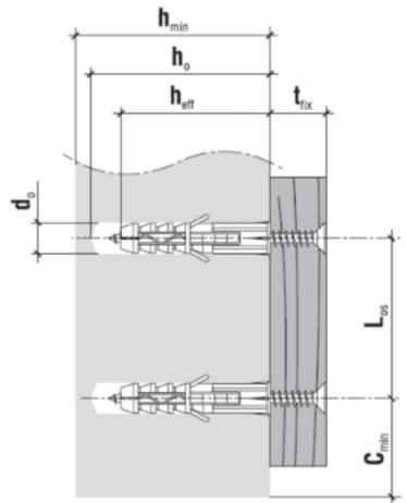
$\begin{array}{l} Hole/drill \mbox{ diameter } [d_o] \mbox{ - 10 mm} \\ Min. \mbox{ substrate thickness } [h_{min}] \mbox{ - 75 mm} \\ Drilled \mbox{ hole } depth \ [h_o] \mbox{ - 60 mm} \\ Anchorage \mbox{ depth } [h_{eff}] \mbox{ - 50 mm} \\ Max. \mbox{ usable length } [t_{frx}] \mbox{ - 20 mm} \\ Min. \mbox{ axial distance (concrete/other substrate) } [L_{os}] \mbox{ - 100/150 mm} \\ Min. \mbox{ distance from edge } [c_{min}] \mbox{ - 100 mm} \\ \end{array}$
