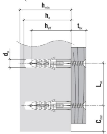
$$\label{eq:hole_drill} \begin{split} & Hole/drill \; diameter \; [d_o] - 10 \; mm \\ & Min. \; substrate \; thickness \; [h_{min}] - 75 \; mm \\ & Drilled \; hole \; depth \; [h_o] - 60 \; mm \\ & Anchorage \; depth \; [h_{eff}] - 50 \; mm \\ & Max. \; usable \; length \; [t_{fix}] - 10 \; mm \end{split}$$
