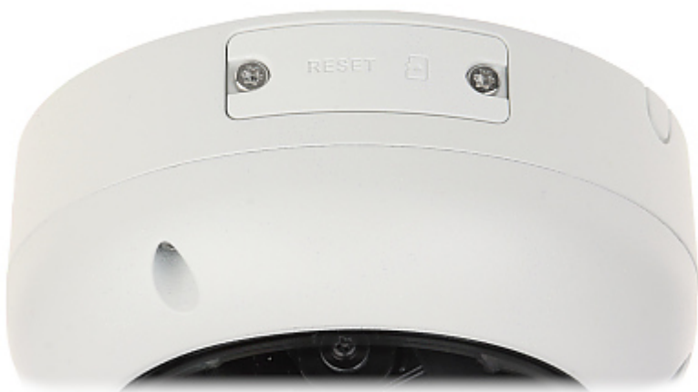
Memory card slot and "Reset" button:
