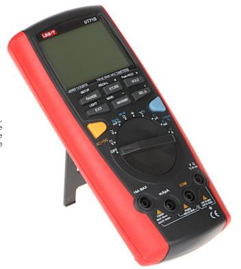
The UT-71D is a universal digital meter used to measure: voltage, current, resistance, inductance, capacitance, frequency, temperature and checking the correct operation of diodes. The meter has the function of automatic change of measuring ranges, as well as the relative measurement mode.
