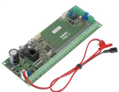
The VERSA-15/EN alarm control panel is intended for security of small and medium-sized facilities, offering comprehensive functionality in the field of security systems. The device has the possibility of wired and wireless extensions, and advanced communication features available through a dedicated GSM/GPRS and TCP/IP communicators.
