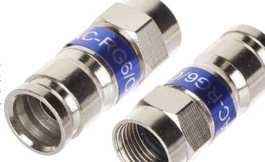
Precise thread eliminates problems with screwing the connectors on sockets. Double compression rings on the cable and the O-ring seal at connection side fully protect the cable and the installation equipment against water penetration.
