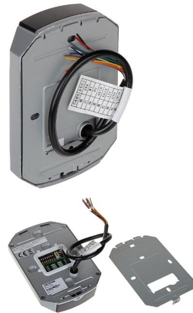
On the body, under the cover there are placed configuration switches:
