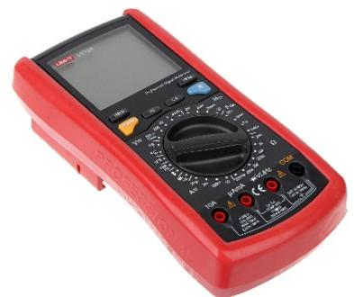
The UT-70A is a universal digital meter used to measure: voltage, current, resistance, inductance, capacitance, frequency, hFE, temperature and checking the correctness of diodes operation.
