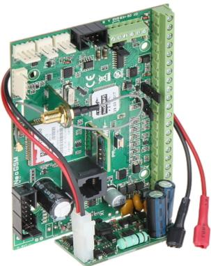
The alarm control panels of NEO-GSM-PS series are intended for security of small and medium-sizes facilities, such as flats, single-family houses, segments in terraced houses, offices, small companies, etc. The control panel in addition to basic, traditional methods of system control
