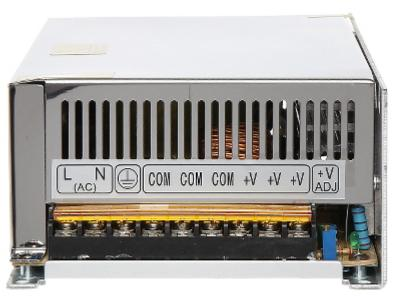
L - Live wire (230V) N - Neutral wire GND - Grounding COM - DC "-" output +V - DC "+" outputs ADJ - Output voltage adjustment
