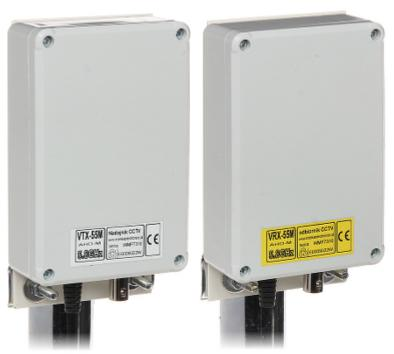
The kit is designed to wireless transmission single video channel of AHD-M / AHD-L / PAL standards in the band of 5.8GHz. It enables radio transmission of the audio and video signals. A both devices have built-in the antennas, which enable good quality transmission up to 300m distance and can operate on the one of the 7 available frequency channels. The channel selection is adjustable by board jumper.
