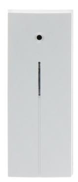
Sensor signals an alarm on registering a low-frequency tone (impact sound), followed by a high-frequency tone (sound of broken glass). The sensor starts to analyze a high-frequency channel after receiving the low-frequency sound wave, caused by the impact.
