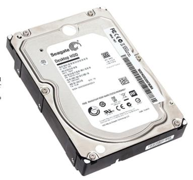
Internal, 3.5" HDD with excellent performance. The high speed of read and write operations allows to use it as sytem disk for daily work. Serial ATA interface connection.
