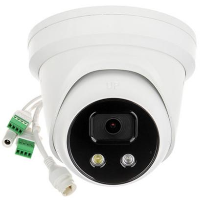
IP camera with efficient H.265 / H.264 image compression algorithm for clear and smooth video streaming at maximal resolution of 6 MPx.
