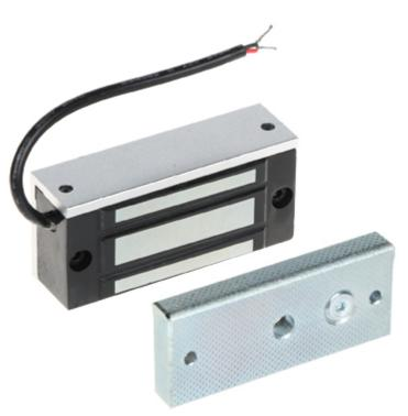
Electromagnetic lock, surface, single. The lock is intended for blocking small wooden, glass or metal doors. Force an entry closed by lock requires the use of force of > 60 kg. It operates reversibly - it is open when power is off. The lock is composed of two elements: electromagnet (usually mounted in the frame) and lock plate (usually mounted in the door). Error free operation of the lock is a result of lack the mechanical elements, which after some time become damaged.
