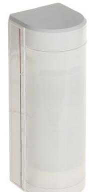
Wireless motion detector, which is designed to detect the moving intruder within the system protected area. With a combination of PIR and MW detection was reached high immunity to false alarms. Thanks to pet immunity, the DS-PDTT15AM-LM-WE can provide protection even when small pets are moving around during surveillance.
