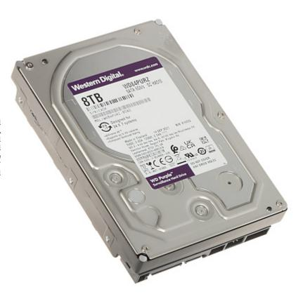
All WD Purple surveillance-class drives are equipped with AllFrame 4K technology, which improves ATA streaming to help reduce frame loss, improve overall video playback, and increase the number of hard drives bays supported within a NVR. These drives are dedicated to HD video recording continuously in 24/7 mode and have reduced energy consumption. Serial ATA interface connection.
