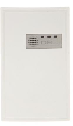
Sensor signals an alarm on registering a low-frequency tone (impact sound), followed by a high-frequency tone (sound of broken glass). The sensor starts to analyze a highfrequency channel after receiving the low-frequency sound wave, caused by the impact. If during this time the high-frequency tone (sound of broken glass) is detected, the detector will trigger an alarm.
