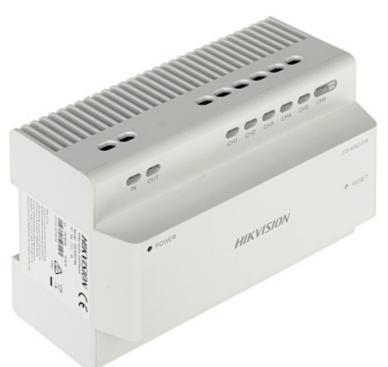
The device has 6 2-wire buses for connecting the monitors and external panels (power supply and signal transmission) and 1 Ethernet socket for connecting the LAN network. In addition, one of the ports is adapted to power an extensive gate station with a maximum power consumption of 16W. In addition, the switch is equipped with additional 2-wire bus outputs for cascading connection with DS-KAD706-S.
