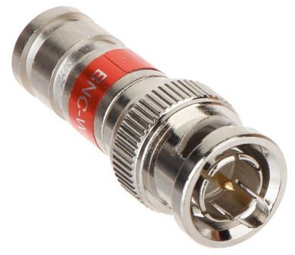
The connector is equipped with a plastic bush, which during compression of the connector is tightly pressed against the sheath of the cable (by putting on cone brass case - the compression ring). The BNC-W/ZAC-RG59/CSR professional compression connector fulfills all recommendations of SCTE (The Society of Cable Telecommunications Engineers) for this kind connectors.
