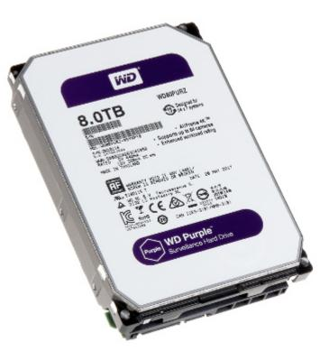
All WD Purple surveillance-class drives are equipped with AllFrame 4K technology, which improves ATA streaming to help reduce frame loss, improve overall video playback, and increase the number of hard drives bays supported within a NVR. These drives are dedicated to HD video recording continuously in 24/7 mode and have reduced energy consumption. Serial ATA interface connection. When you purchase the HDD with DVR, the HDD montage into DVR and operating tests are free of charge.
