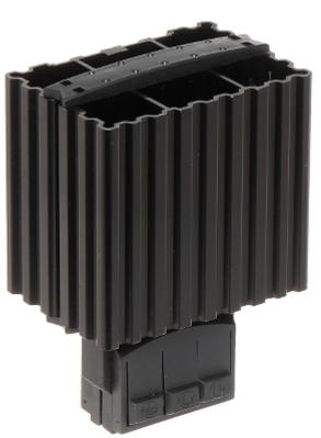
The HG-140-15W semiconductor heater operates based on a PTC thermistor. Heaters and fan heaters prevent condensation of water vapor and maintain the proper operating temperature of the devices. For optimum circulation of air it is advisable to install the convection heaters in the bottom part of the cabinet in a vertical position.
