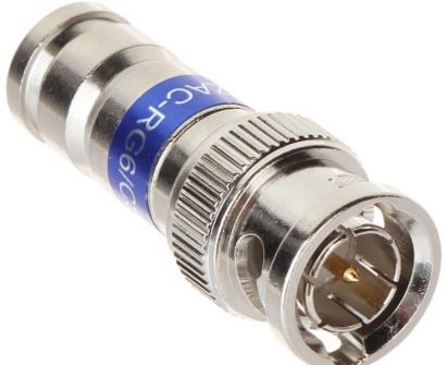
The connector is equipped with a plastic bush, which during compression of the connector is tightly pressed against the sheath of the cable (by putting on cone brass case - the compression ring). The BNC-W/ZAC-RG6/CSR professional compression connector fulfills all recommendations of SCTE (The Society of Cable Telecommunications Engineers) for this kind connectors.
