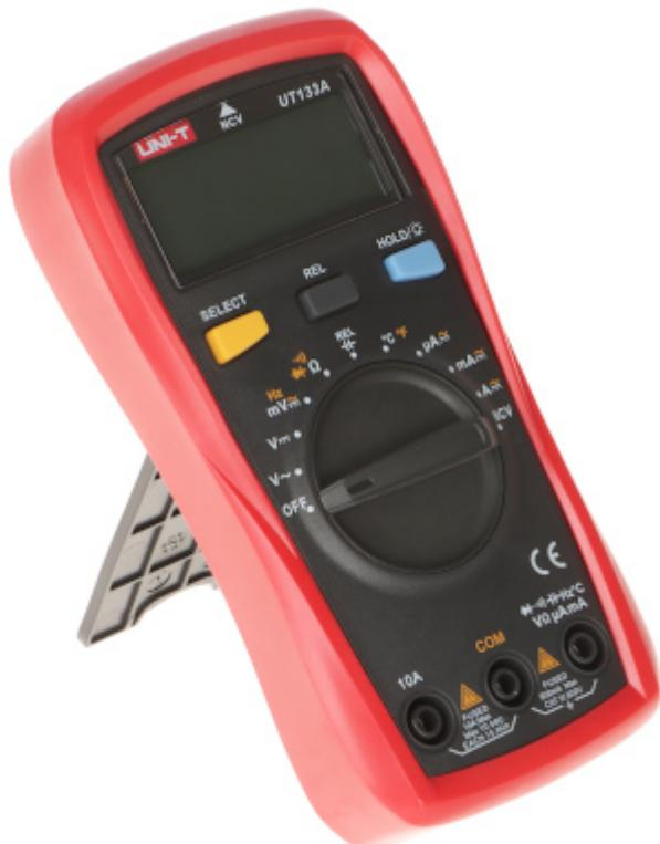
The UT-133A is a universal digital meter used to measure: voltage, current, resistance, capacity, frequency, temperature and checking the correct operation of diodes. The meter has the function of automatic change of measuring ranges, as well as a relative measurement mode (when measuring voltage, current and resistance).
