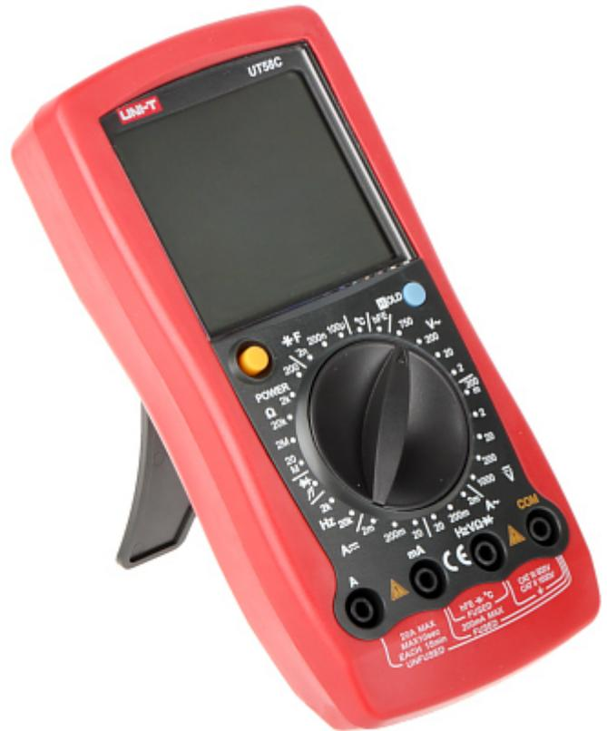
The UT-58C is a universal digital meter used to measure: voltage, current, resistance, capacitance, hFE, and checking the correct operation of diodes.
