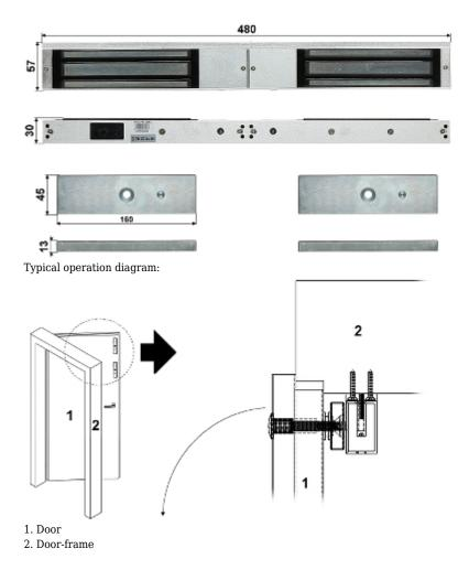
Should pay attention to rubber pads mounted between the door and the movable element of the lock. These pads ensure proper fit the lock elements with the door when it is closed.
