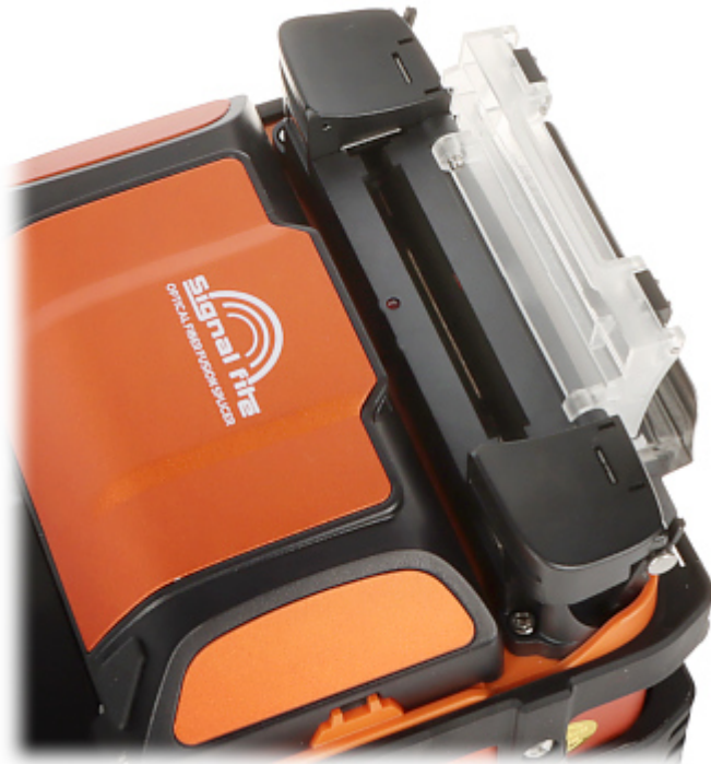
A heating oven for heating the splice sleeves:
