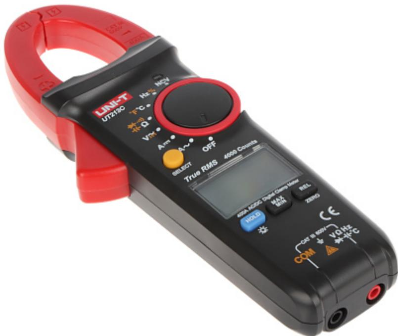
The UT-213C is a universal digital meter equipped with clamps enabling the measurement of high currents. The device measures: voltage, current, frequency, resistance, capacity and temperature. In addition, the meter has an electric field detection function (NCV).
