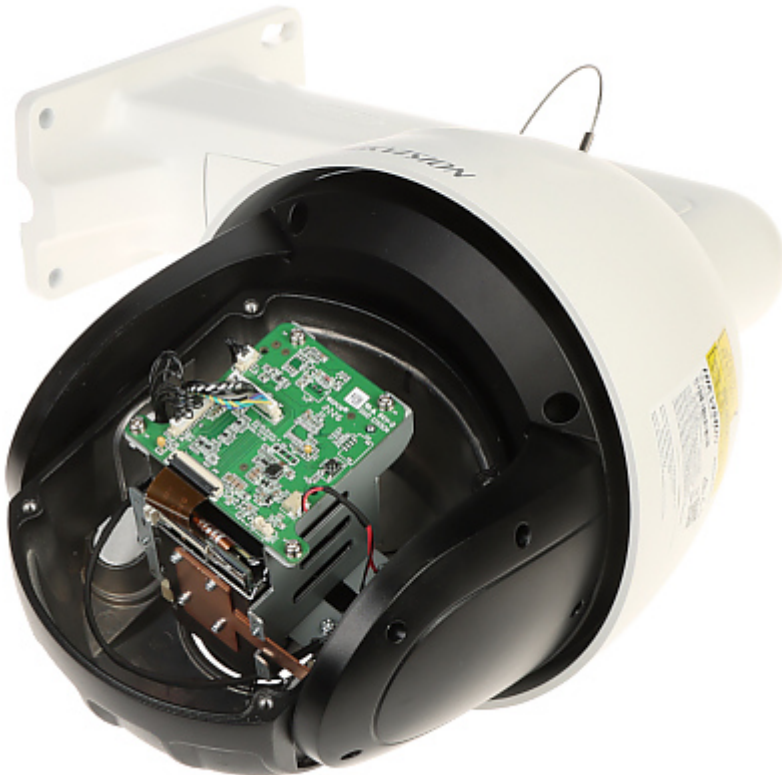
Micro SD card slot is located inside the camera:
