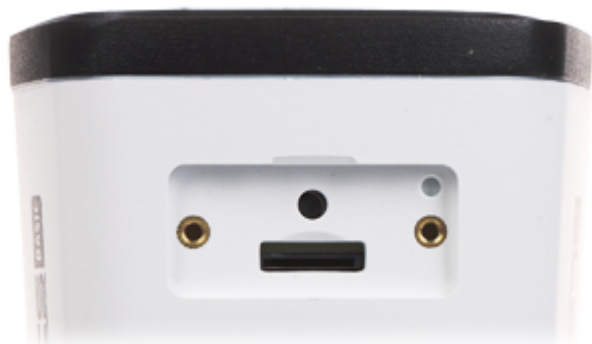
Memory card slot and "Reset" button:
