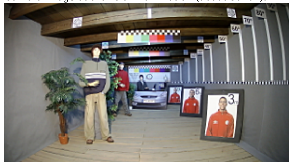
Camera image at artificial illumination (about 30Lux):
