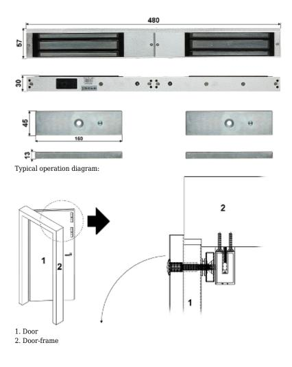
Should pay attention to rubber pads mounted between the door and the movable element of the lock. These pads ensure proper fit the lock elements with the door when it is closed. In the kit:
